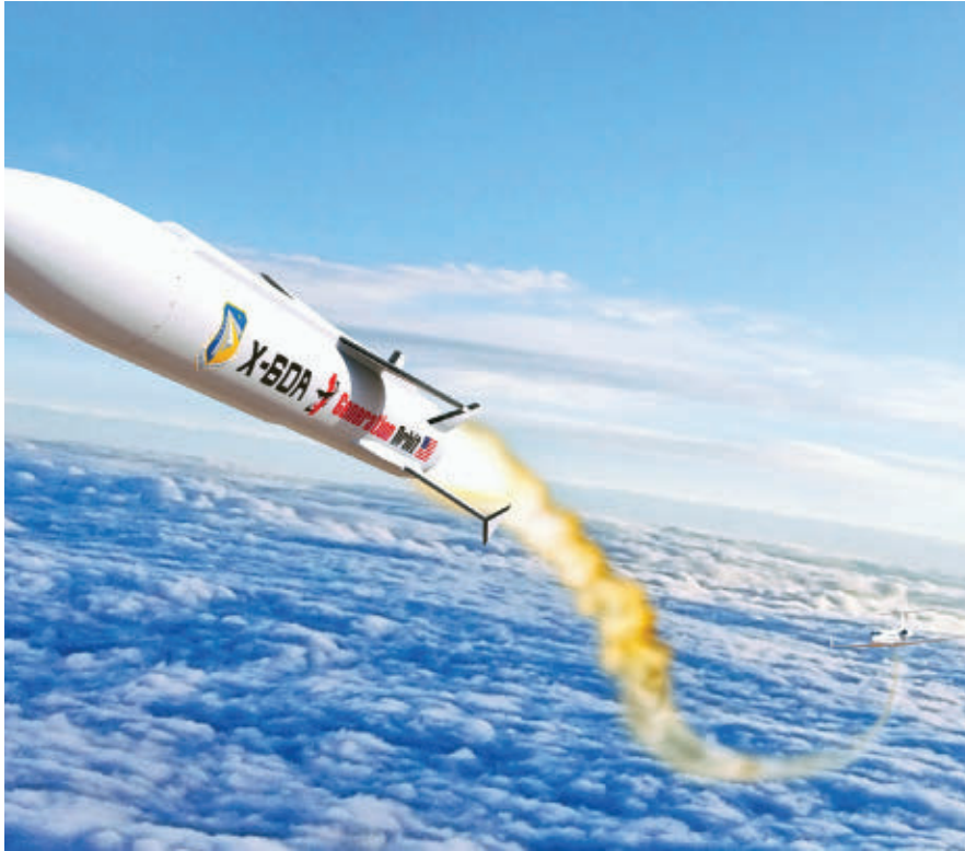
The Generation Orbit X-60A project seeks to develop an affordable launch and propulsion system that could be applied to future hypersonic munitions and vehicles.
