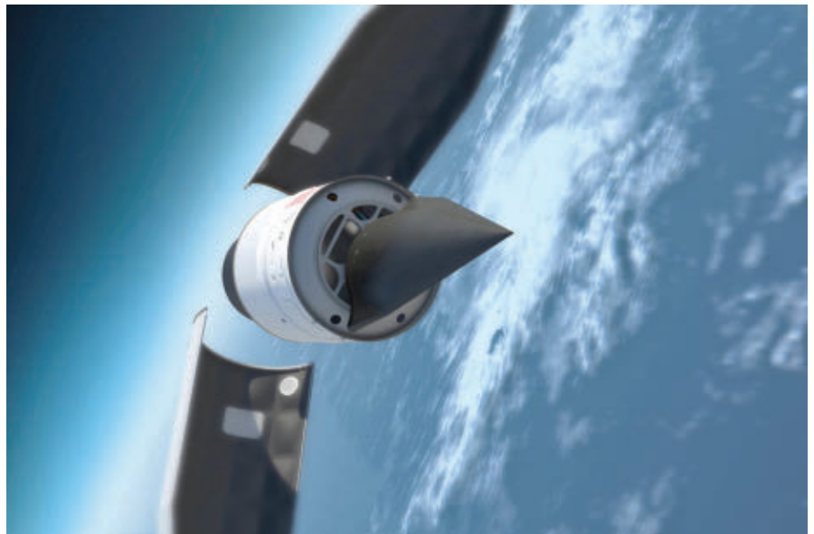
The DARPA Falcon Project seeks to develop a reusable, rapid-strike hypersonic cruise missile, as well as a launch system to accelerate the weapon to hypersonic cruise speeds.
