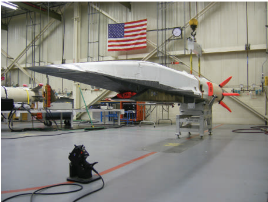
The X-51 Scramjet Engine Demonstrator, called Waverider, flew four times between 2010 and 2013 to prove the viability of a scramjet-powered vehicle for hypersonic weapons applications.
